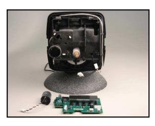
Unhinge the drive bracket by using the two finger tabs on the top left and top right of the black drive bracket – then thread the power cable into the valve and attach to the connection marked 12 VAC on the green PC board.
